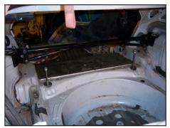
**Step 7:** Prior to installing the lower floor/subspace frame support you must thread the 9" long steel rods completely flush with the subfloor.
